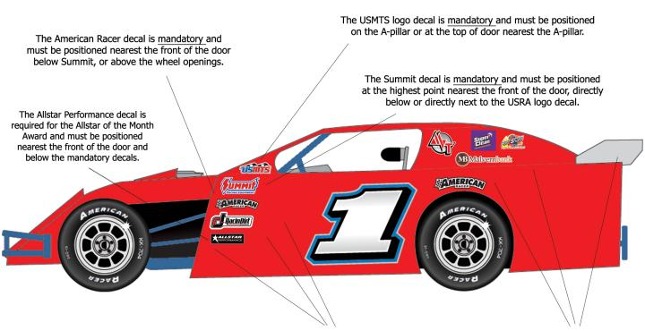
The Fast Shafts, Malvern Bank, MVT, RacinDirt and Super Clean decals must be positioned on the outside of the body or the sail panels.
